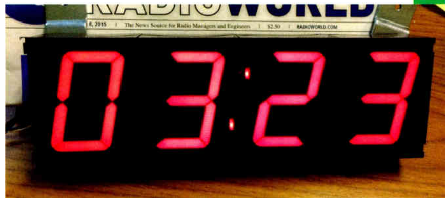
Fig. 1: Bruce Roberts uses a large 2-1/4-inch clock module to time talk segments.
