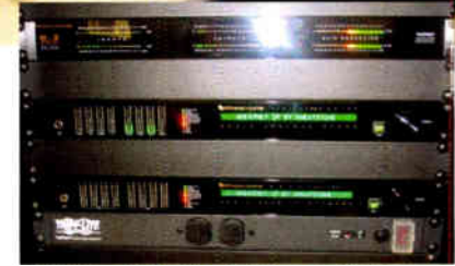
Shown is web radio OWWR's number-one studio with IP-12 control surface, M-2 dual mic processor, and just the right amount of WheatNet-IP audio networking. Check out those baby-proof covers on the Tripp-Lite power module!
