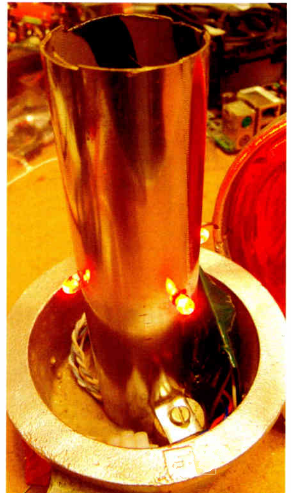
Fig. 5: The LEDs are mounted to a piece of chrome sink drainpipe.
