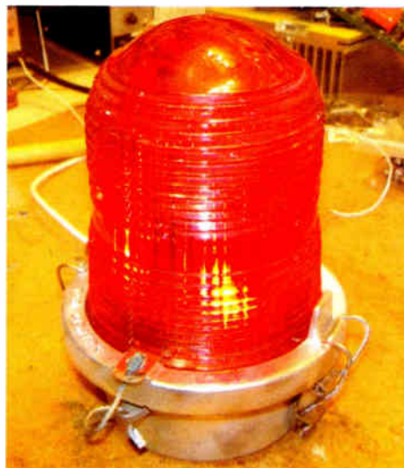
Fig. 4: Mount the flasher in an old tower side-lamp fixture.
