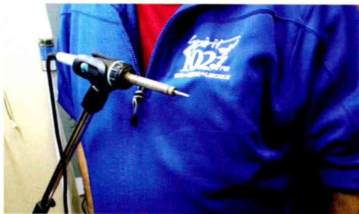
Fig. 6: Use a floor mic stand to hold a soldering iron inside a rack.
