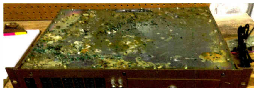
Fig. 2: Rodents can do great damage. Mice nearly ruined this processor.
