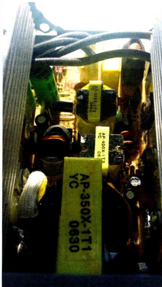
Fig. 1: It's not over 'til the fat PSU "sings." Cheaply-built PC power supplies can be a source of mystery mechanical noise.
