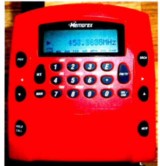
The clean, neat, organized dashboard of Scannocular makes it a snap to program. Note the old TV (FM/TV) band button.
