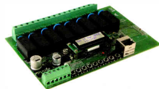
Fig. 3 Velleman's VM201 Ethernet relay card can be controlled by a smartphone.
