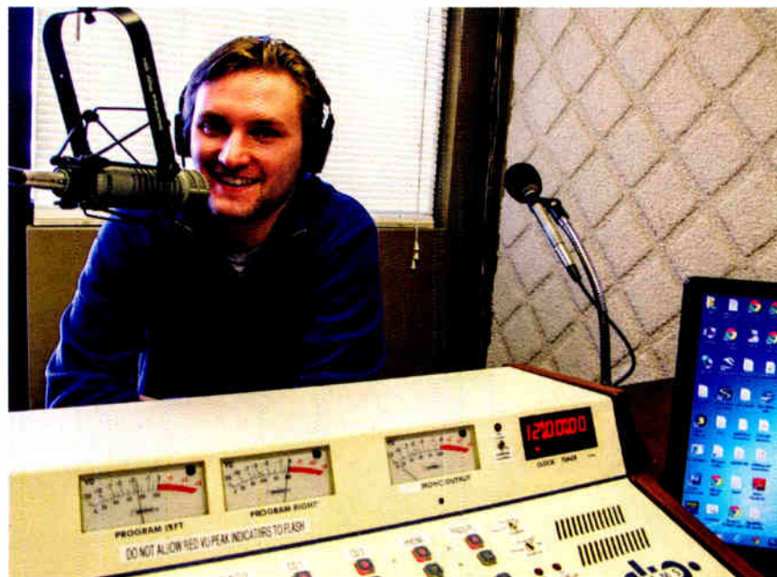
Fig. 1: Note the 3 dB difference in left- and right-channel levels shown by the console VU meters in this photo of announcer Pete Vukelich in the studio of WWWW Radio in Baxter, Minn.
