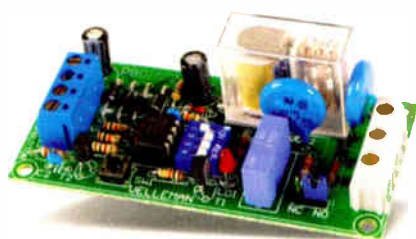
Fig. 1: The Velleman K8015 is a multifunction relay kit with adjustable delay.
