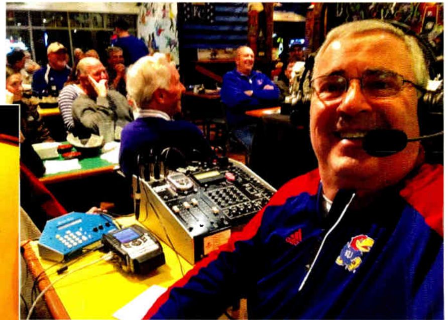
Bob Newton at a remote with his gear, including a Comrex Access codec and an older piece, a Comrex BlueBox codec.
