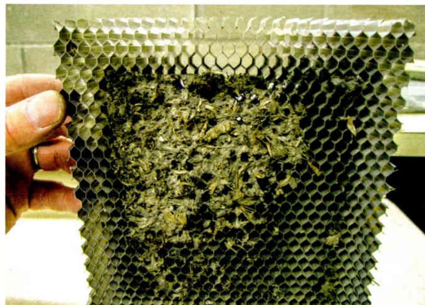
Fig. 2: A clogged honeycomb air filter from a Continental FM transmitter.
