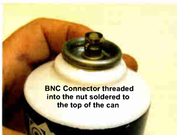
Fig. 7: Thread the BNC connector and stub assembly onto the nut.
