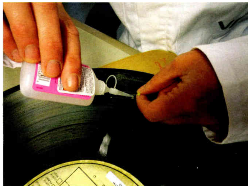
Operators wash a lacquer disc with ammonia.
