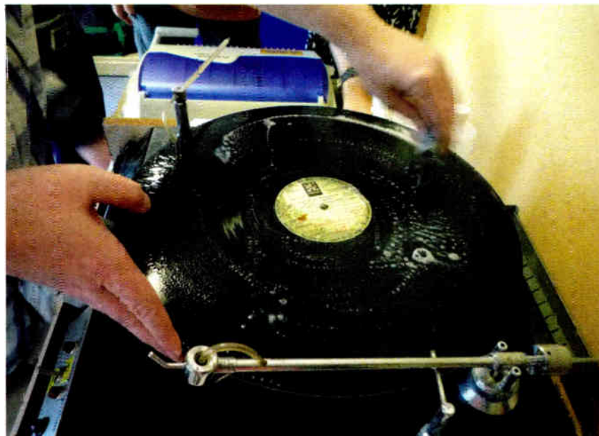
Each side of every record is washed with osmosis water, ammonia, nonalcohol-based detergent or lamp oil and, if necessary, repaired with additional wax or glue.
