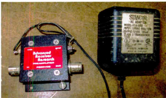
Fig. 6: An STL preamplifier with a problem.
