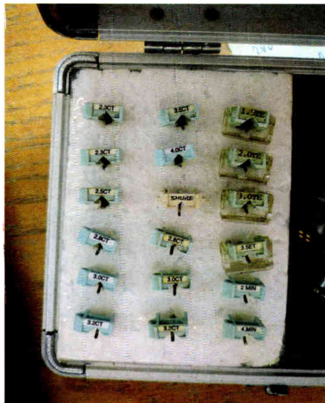
The VRT's stylus vault for the digitization project. A specific needle is available for each type of record.
