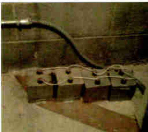
Fig. 1: Stringing a few capacitors together got the transmitter running.
