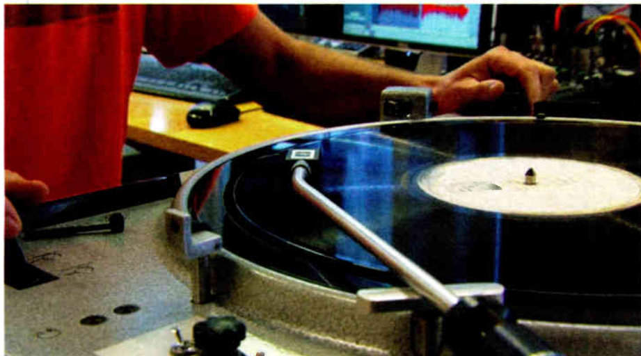
A lacquer disc is played on one of VRT's vintage EMT 921 record players equipped with a dedicated stylus.
