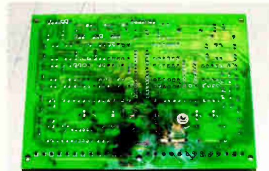
Fig. 4: The lightning also vaporized traces on the control board.
