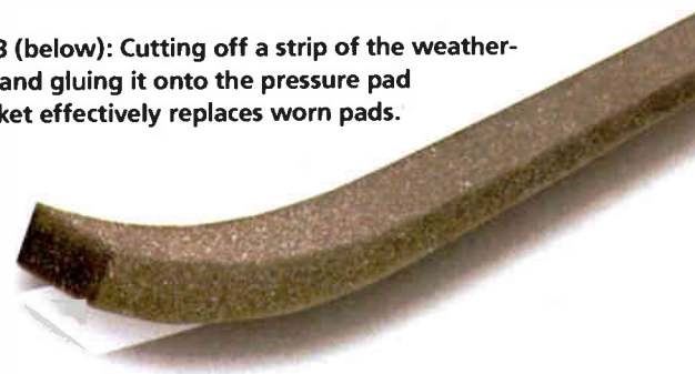
Fig. 2 (left): A roll of foam weather-seal works for pressure pad replacement.
