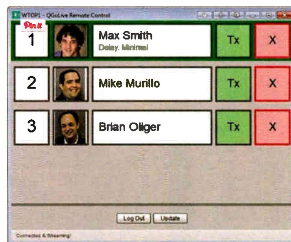
A remote control app lets the producer see who's connected to QGoLive and manage who's on the air. Connected users hear the reporter on-air.
