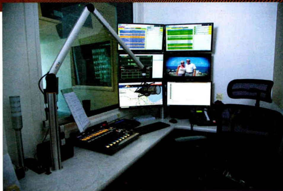
One of the three call screener/producer studios, each with direct line-of-sight into its associated air studio.
