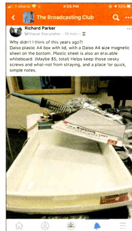
Fig. 3: An inexpensive document tray with a plastic lid, from Daiso Japan, holds parts while equipment is being repaired.
