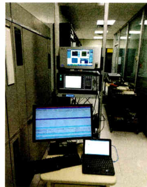
Left and above: An RFmondial reference receiver is shown with a Transradio DMOD3 DRM exciter and an RFmondial Livewire audio router. The large screen is the user interface for a 1RU content server situated behind the screen.
