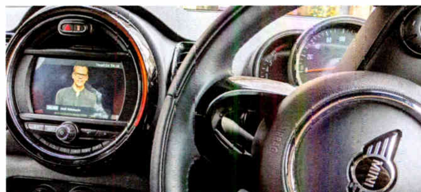
Here's the view for a U.K. driver of a recent model Mini. The screen at left shows visuals created by Heart London that have been transmitted via DAB digital radio.
