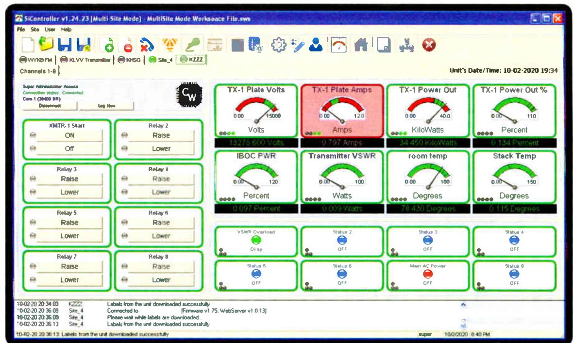
Remote control systems are tasked with managing increasingly complex site networks. Shown is a CircuitWerkes Sicon-8 system in multisite mode.
