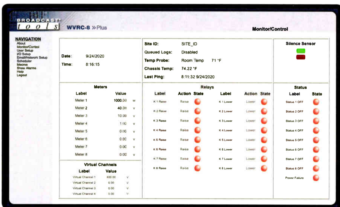
The HTML-based monitor and control web page of a Broadcast Tools WVRC-8 Plus remote control.
