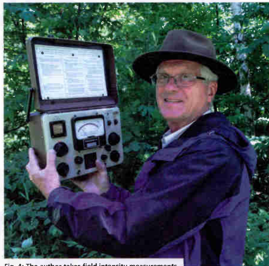
Fig. 4: The author takes field intensity measurements.
