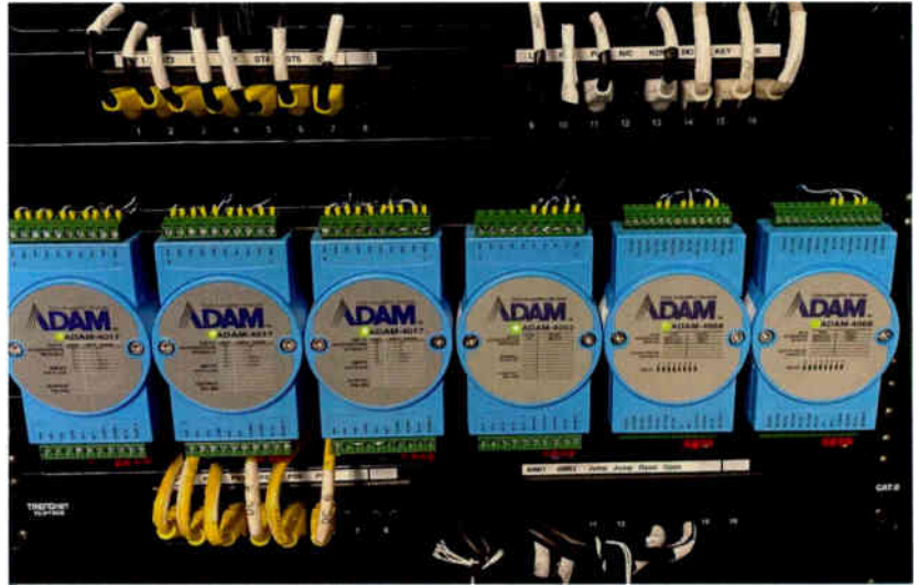
Above A Stellar Eclipse site monitor and protection system with VSWR Sentinel is shown serving four FM stations and their shared antenna and combining systems.
