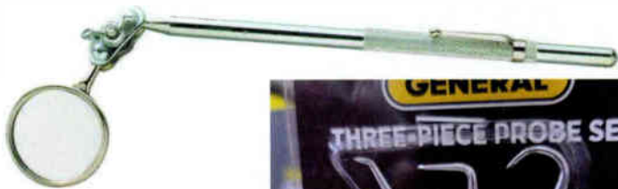
Above Fig. 3: A small inspection mirror gets into tight spaces.
