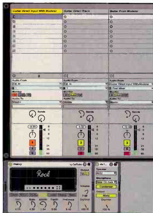
An input channel with plug-in (left) feeds recording track (right). A direct track (center) simultaneously captures guitar straight from the interface.
