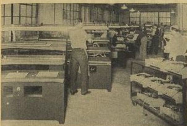
A BUSY DEPARTMENT in the big O. D. Jennings & Company plant is the cabinet assembly department for telephone music units. Highly skilled workers are entrusted with the work of assembling the most important part of the system.
