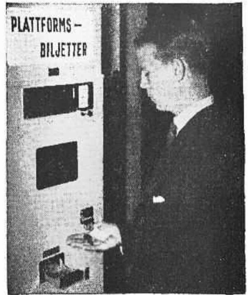
COIN SLEUTHING is a feature of this Swedish railway ticket vending machine, on location at Stockholm Central Station. Besides vending tickets and making change, machine includes concealed camera which snaps picture when slug or counterfeit coin is inserted, photographing offender in the act. Meaning of Plattform-Biljetter: Platform-Tickets.
