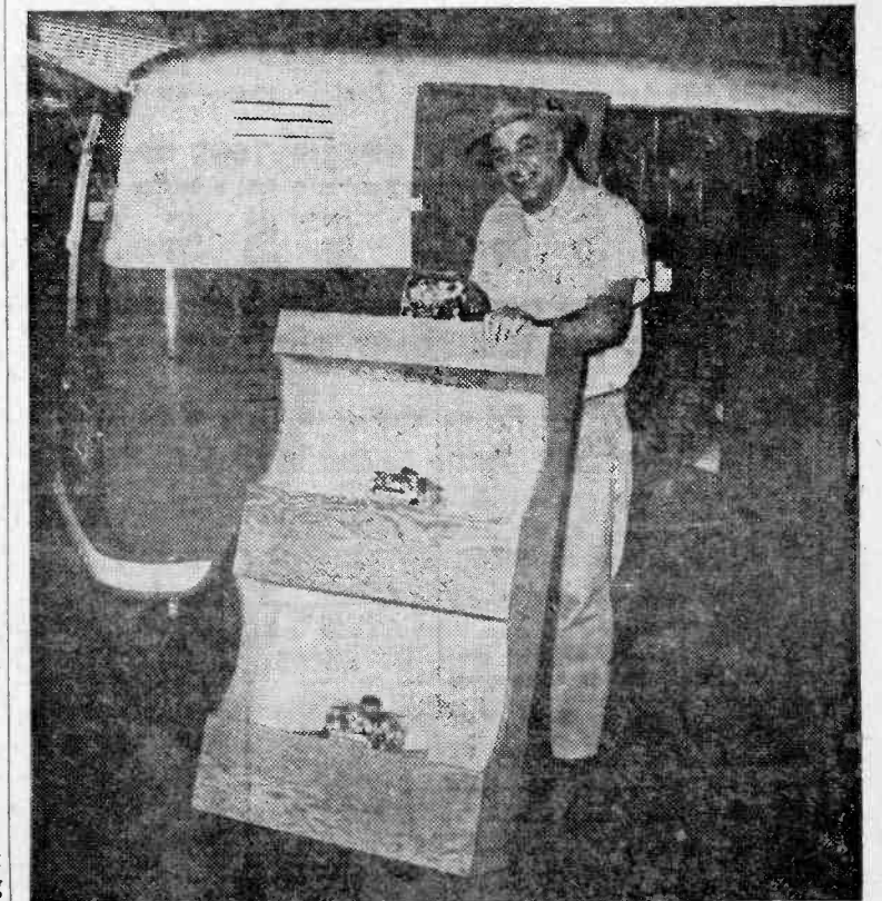
THIS BOX-LIKE AFFAIR holds nine pre-filled heads and saves Joe Arguelles a lot of steps. The box is secured to the light-weight aluminum dolly with a bolt and butterfly nut.
