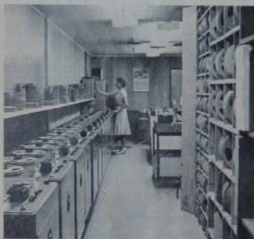
THE DUPLICATING ROOM where 10 custom-built Ampex duplicators handle the high volume of taped programs sent to thousands of customers throughout the world.
