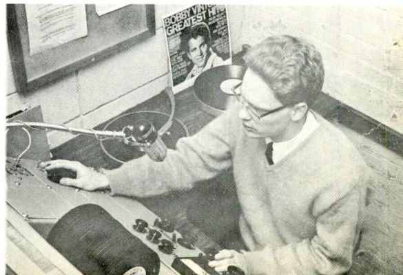
Jack Ekwall, station engineer, airing a show. Control board is designed for combo operation—does not require an engineer on duty.
