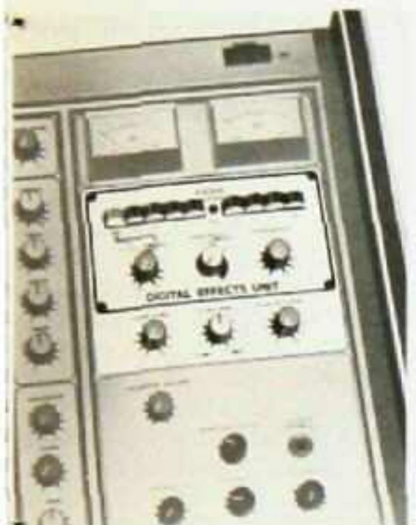
CCD Echo Effects module for HH Electronics' Stereo 8 and Stereo 12 mixers via U.S. distributor Audio-marketing offers pushbutton echo, reverb, flanging, vibrato and phasing sound effects.
