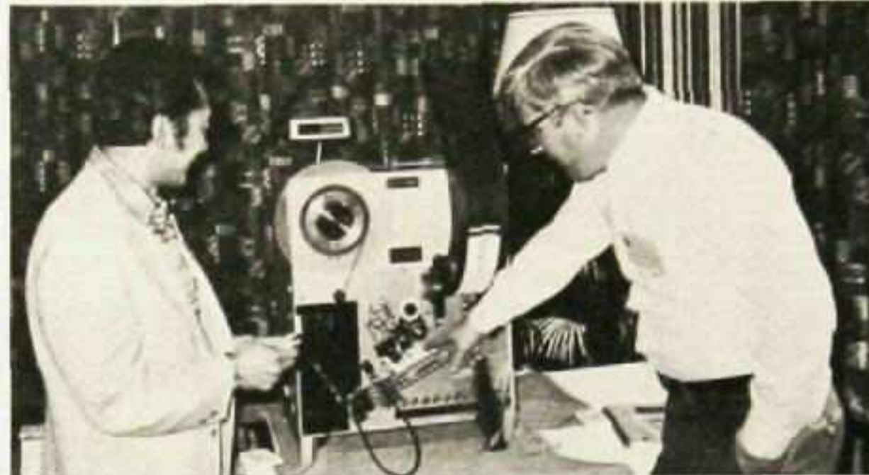
KING Instrument's Bill Cline, right, points out special features of the latest model 760 high-speed self-feeding automatic cassette loader to Mort Fujii of Cetec Audio. King also recently introduced a new videocassette loader than can handle both Beta and VHS-format shells.
