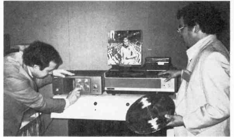
DIRECT DISC's Joe Overholt, left, adjusts PCM adaptor for digital U-Matic cassette recording used to back up direct disk master of new "Power" release held by firm's Dave Lintz. Label plans release of first PCM digital cassettes in fall.
