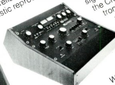
GLI Model 1000 signal processor and 3880 mixer/preamplifier mounted in WC-1 cabinet.
