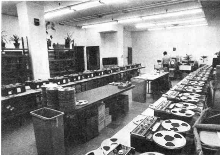
Slave Room: Symphony and opera performances are duplicated in one-to-one ratio on 30 Revox "slave" machines at the WFMT-FM facility. The duplicating operation is one year old.
