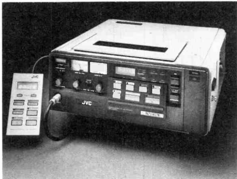
PRO VIDEO —JVC's CR-4700U portable professional videocassette recorder features a separate pair of playback heads that scans the videotape just 8.3 milliseconds after the video track is recorded, permitting instant video preview. Another feature is SMPTE time code capability.
