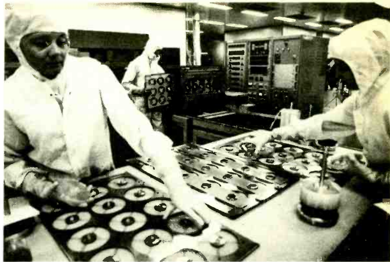
FRESH OUT OF THE OVEN—Employees at the newly opened CBS/Sony Compact Disc plant in Terre Haute, Ind. place a thin layer of aluminum over the mold's pitted surface which reflects the CD player's laser.
