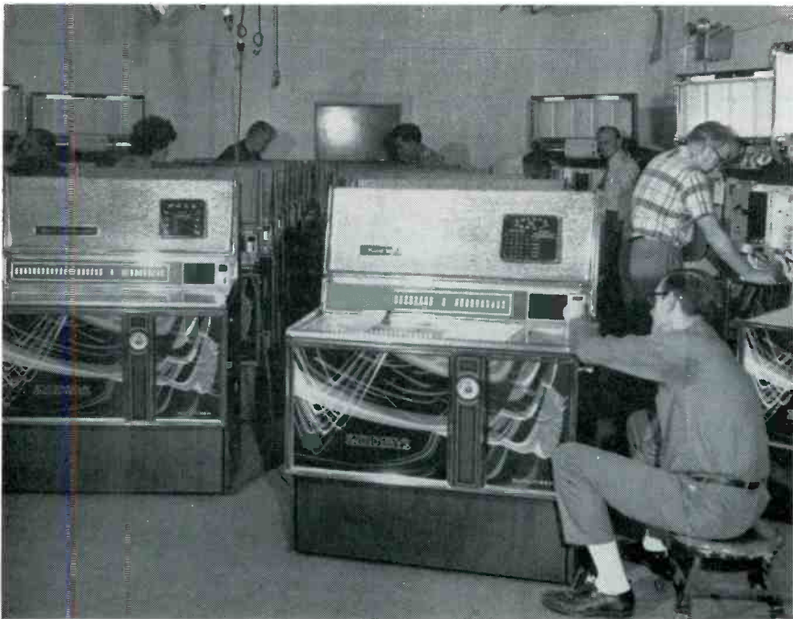
Technicians at the Wurlitzer North Tonawanda, N.Y. factory carry out one of the final stages of production of the new "Zodiac" phonograph. In the above production view of the final test and check out section in quality control, various models of phonos with 100, 160 and 200 selections are shown receiving approval prior to shipment.
