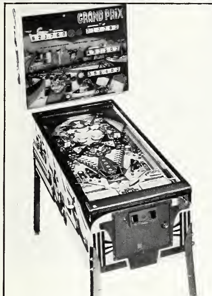
GRAND PRIX — Williams Electronics Inc. premiered its Grand Prix pinball game at last year's AMOA Expo. Scoring features on this four-player game include left and right bonus lanes with spinner units for 1,000 points; left and right center kick-out holes for bonus; advance bonus rebound rubbers and drop targets that light one to four stars (number two star scores an extra ball and number three star a special). The game is encased in a colorfully illustrated cabinet with car racing graphics.
