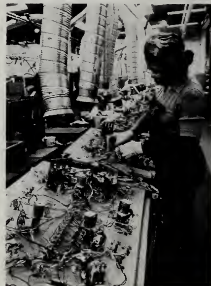
Pictured above is the playfield assembly line at the Williams Electronics factory.
