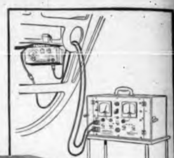
Diagram, above, shows how the Conn Interval and Dwell Tester (left) is "hooked-up" to a B-24 for checking accuracy of Bomb Release Interval Control on plane before bombing mission.
