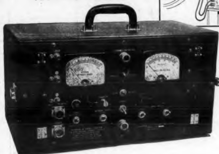
Diagram, above, shows how the Conn Interval and Dwell Tester (left) is "hooked-up" to a B-24 for checking accuracy of Bomb Release Interval Control on plane before bombing mission.
