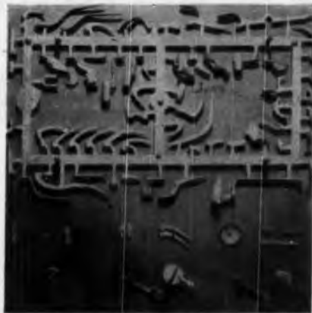
One set of 35 alto-sax keys cast at one operation. After 1100 other manufacturing operations, a finished set of keys results.
