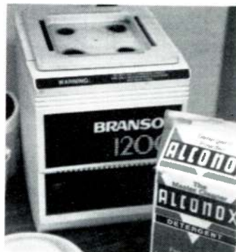
Ultra sound cleaning machine and laboratory detergent used for cleaning, prior to sterilization (courtesy of Tattoo Mania).
