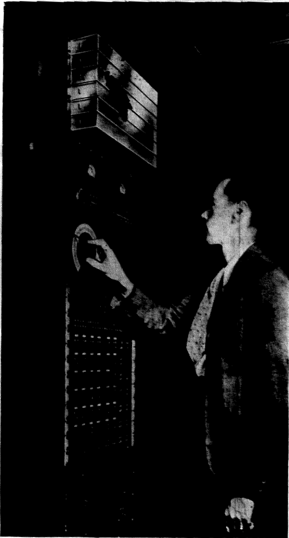
The Type 52-B Oscillator on the master control racks of the Amalgamated Broadcasting System, New York City.
