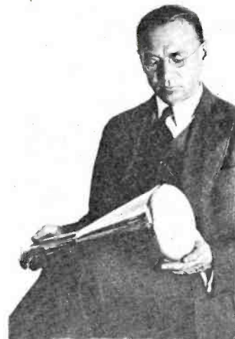
THE "KINESCOPE"—Heart of the RCA's television receiving system, on the white convex surface of which its 343-line pictures are built up and framed at the rate of 60 per second. Dr. Vladimir Zworykin is shown holding the tube.
