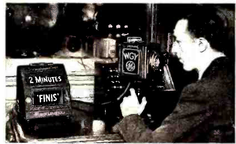
TIMER—This electric gadget warns speakers at WGY, Schenectady, of the two-minute line and the conclusion of his speaking period. It may be set for any time up to 30 minutes, a telechron motor operating a set of switches which in turn operates relays. A tone chime can be used with the "finis" warning.
