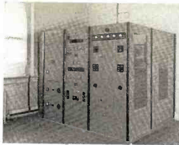
REL 1 kw FM transmitter at W3XO—Washington, D. C.—Jansky and Bailey—in operation since August 1939.
