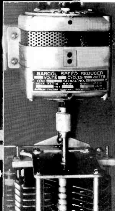
This is a close-up of the motor used to tune the final grid circuit. Considerably more power is available than is necessary to assure smooth operation at all times . . .
