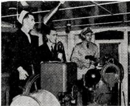
WHEELHOUSE on the bridge is ship's "brain." The "talker" at left relays a command of the Executive Officer Lt. Cmdr. A. W. Beale to the lookouts. The quartermaster, or helmsman, mans the wheel. At left is the engine room telegraph; at right, the ship's gyro-compass.
