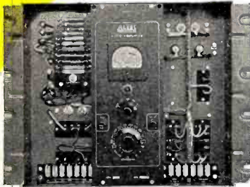
ALTEC LANSING A255 AMPLIFIER Power Output: 35 watts —Gain: 65 DB • Frequency Range: 20 to 20,000 cycles.
