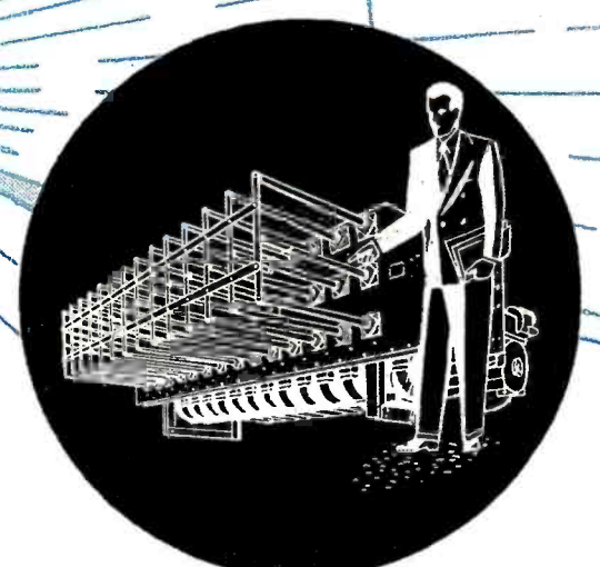
1941 Polyrod radar antenna was an important war contribution ... helped sink many Jap ships. Its exceptionally narrow beam and rapid scanning gave high accuracy to big Navy guns.
