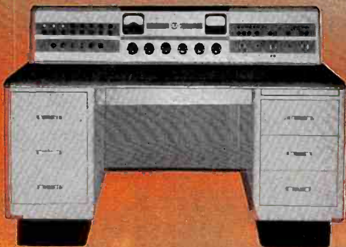
CONTROL CONSOLE contains controls for both the transmitter and audio channels. Every major function of the transmitter is at the engineer's finger tips or within easy viewing distance.
