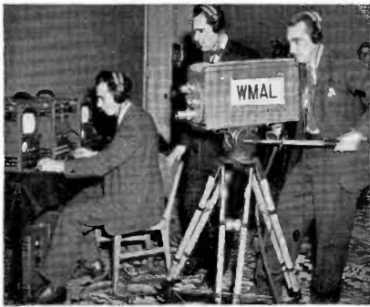
To gain valuable operating experience prior to on-the-air service, WMAL for many months has been using RCA image-orthicon field equipment for experimental pick-ups.
