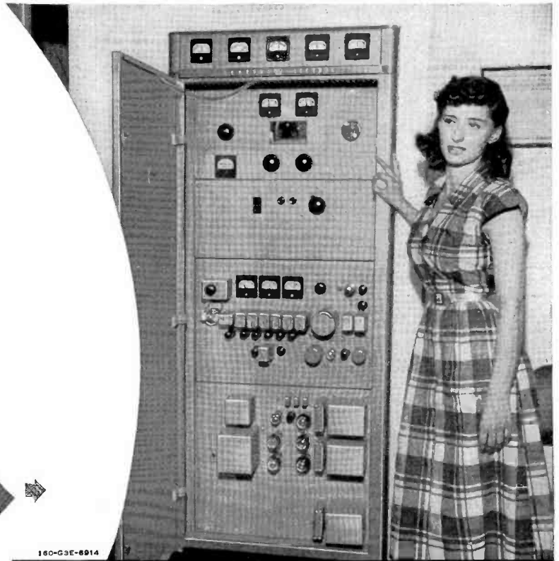
Radio Intercom at network headquarters in Ithaca is powered by 50-watt G-E wall-mounted transmitter. From here studio officials enjoy two-way communication with 5 jeep crews and all stations of the net. Sturdy, dependable intercom eliminates problem of party line phone service in rural areas.
