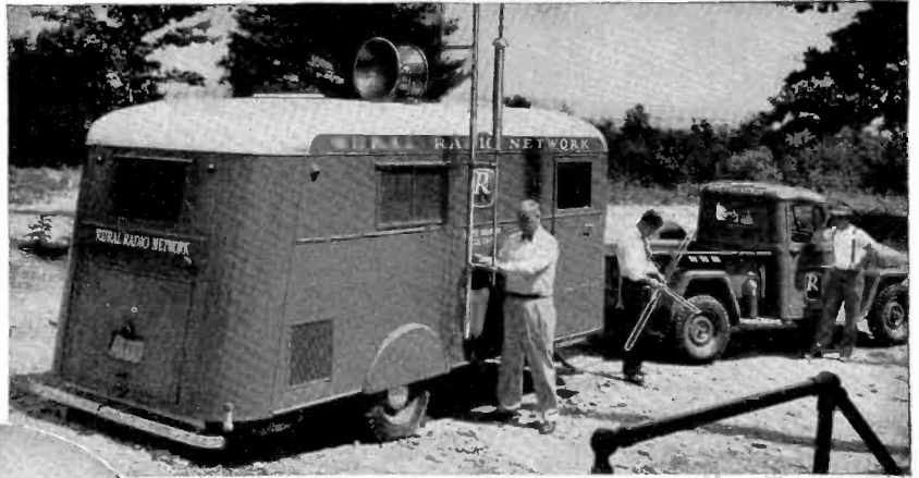
Mobile Unit —hailed by jeep, covers county fairs, livestock shows, can broadcast from virtually every back pasture in the state. Completely G-E equipped, truck contains 50-watt transmitter which feeds remotes into network at any point, plus wire recording apparatus, amplifiers and all accessory items. Two-way radio in jeep also ties into network intercom.
