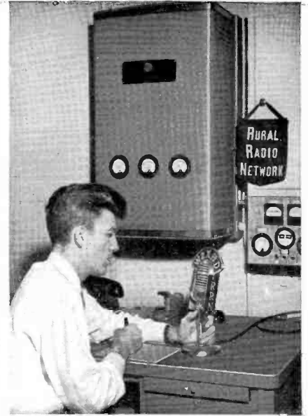
Radio Intercom at network headquarters in Ithaca is powered by 50-watt G-E wall-mounted transmitter. From here studio officials enjoy two-way communication with 5 jeep crews and all stations of the net. Sturdy, dependable intercom eliminates problem of party line phone service in rural areas.
