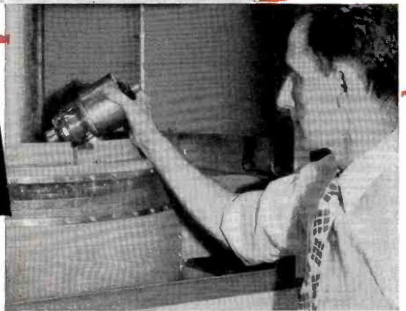
TUBE COSTS SLASHED: Lightweight, air-cooled triodes are used exclusively in the "Symmetron" FM amplifier.
