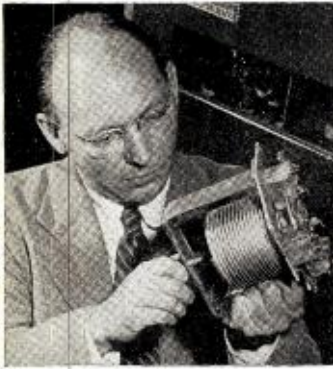
RCA ENGINEER demonstrates the tuning process of the new 500 w television transmitter, now in production by the RCA Engineering Products Department.
